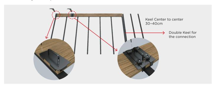
**STEP 2**Both screw positioners keep a **3mm** space between the decking boards.
